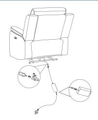
Safety Note: Transformer and cables are not to be placed under or within the recliner structure.
